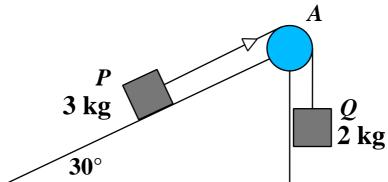
Two particles *P* and *Q* of masses 3 kg and 2 kg respectively are connected by a light inextensible string. Initially *P* is held at rest on a fixed smooth plane inclined at  $30^{\circ}$  to the horizontal. The string passes over a small smooth pulley *A* fixed at the top of the plane. The part of the string from *P* to *A* is parallel to a line of greatest slope of the plane. The particle *Q* hangs freely below *A*. The system is released from rest with the string taut.
