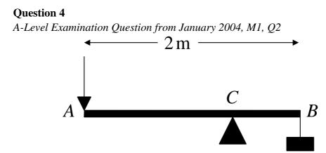
A lever consists of a uniform steel rod AB, of weight 100 N and length 2 m, which rests on a small smooth pivot at a point C of the rod. A load of weight 2200 N is suspended from the end B of the rod by a rope. The lever is held in equilibrium in a horizontal position by a vertical force applied at the end A, as shown. The rope is modelled as a light string.
